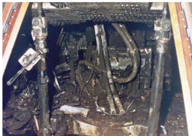
A close-up view of the interior of the Command Module shows the effects of the intense heat of the flash fire.
